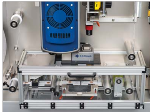
Shown with laser printer and code presence verification camera options
